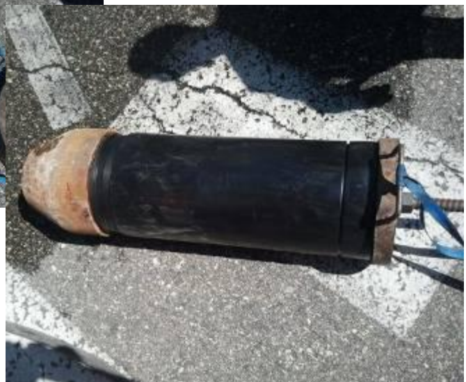
↓ The calibre head Ø 295 mm (11.6") with short pipe OD 280 x 10.7 mm (OD 11.0" x 0.42"), pressure plate and pipe rod.
