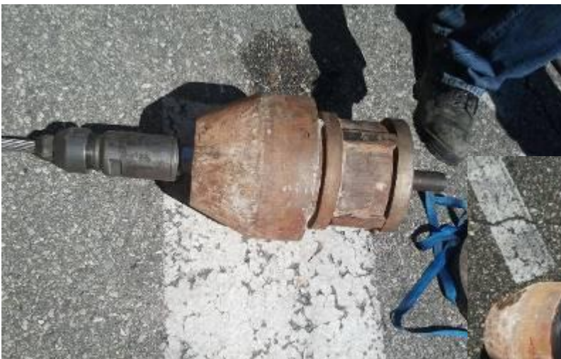
↑ The calibre head is connected with the cable coupling to the pulling cable of the cable burster X 400.
