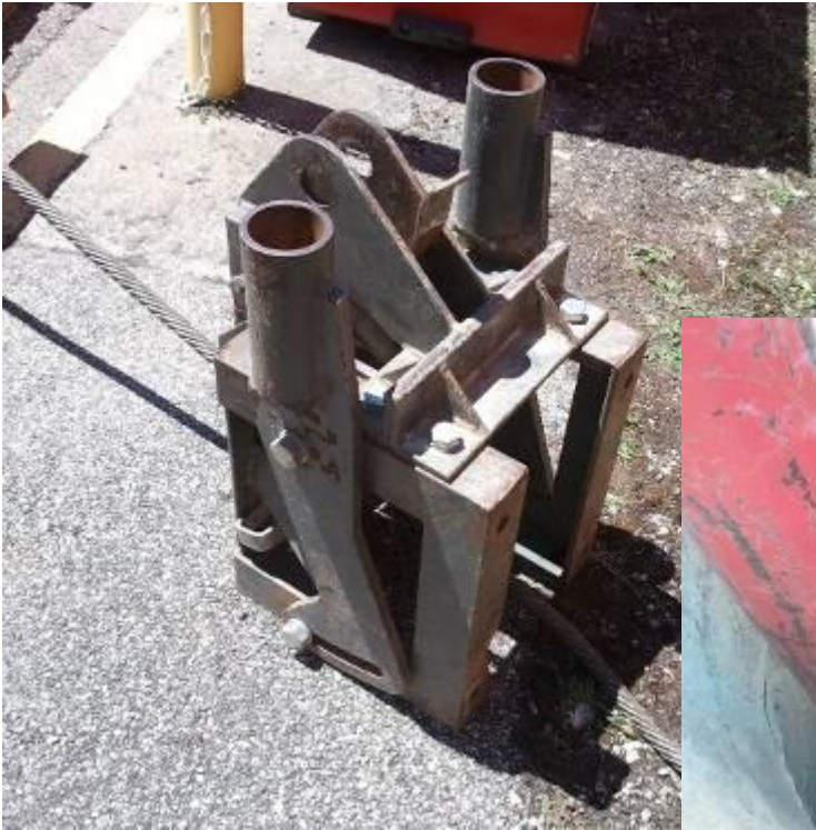
↑ This manhole frame fits through the manhole opening Ø 620 mm (24.4") and can be positioned into manholes Ø 800 mm (32") and 1'000 mm (40").
