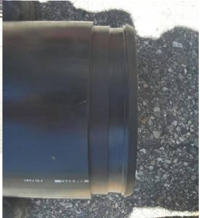
↓ The positively locked plug connection with seal and notch.
